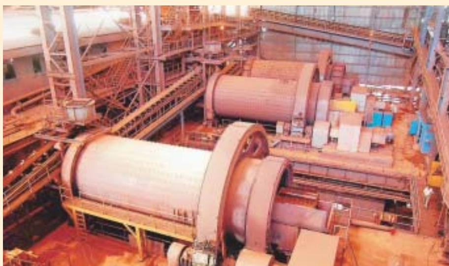
Wet grinding environment friendly technology adopted for the first time in KIOCL for processing Hematite Grade Ore from the Bellary Hospet Region.
