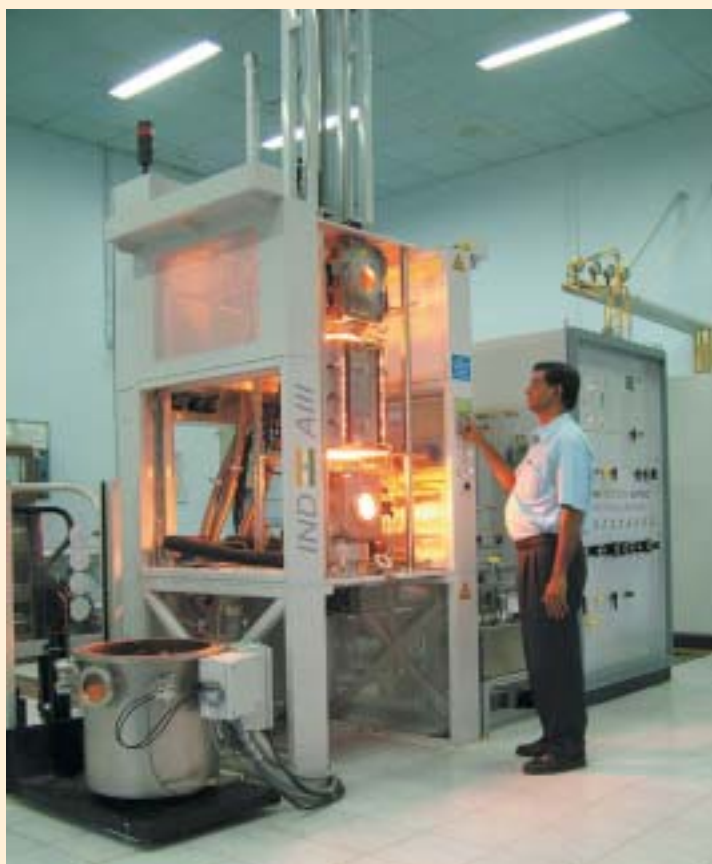
Experimentation in Hot Dip Process Simulator at R&D Centre for Iron Steel (SAIL) for ensuring best quality products.
