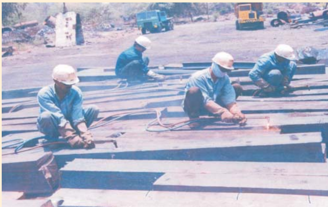
Processing of Mill rejects through gas cutting operations by FSNL, at Bhilai Steel Plant.
