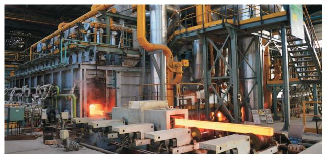
Special Bar Mill of capacity to produce 7.5 lakh tons per annum of plain rounds in straight length and in coil form with free size rolling for customized sizes commissioned at RINL
